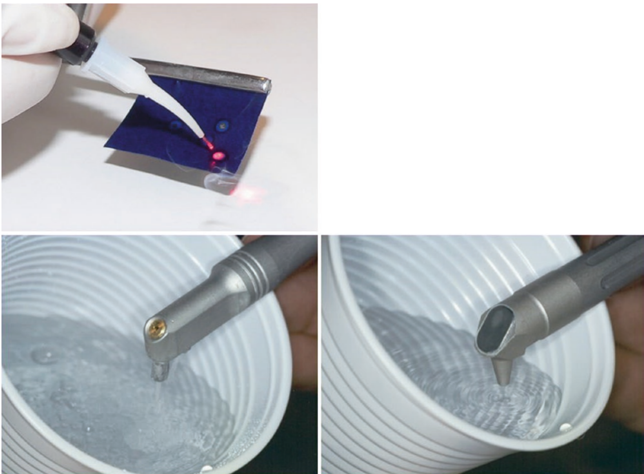
Fig. 5.4 Laser test fire. Using minimum laser operating parameters, the beam is directed into a suitable attenuation medium. Top center, for visible and NIR wavelengths pigmented articulating paper. Bottom left, water for (mid-IR) Erbium YAG; bottom right, water for CO 2 wavelengths
