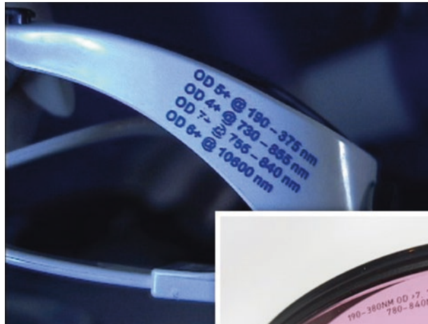
■ Fig. 5.6 Examples of laser safety eyewear, with relevant optical density (OD) values applicable to specific wavelengths. OD scores of 5.0 and above are considered explicitly safe in protecting the wearer's eyes. This information may be found on the eyewear lens or on the sidebars
