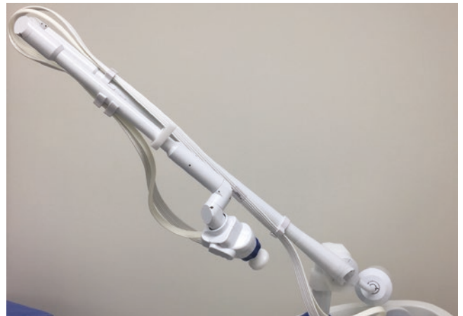
■ Fig. 2.7 An articulated arm delivery system
