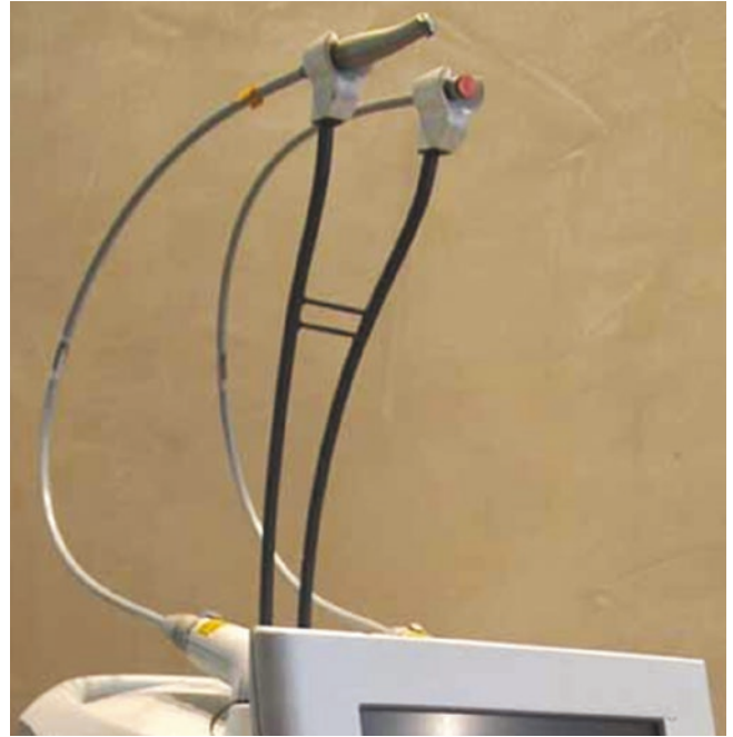
■ Fig. 2.6 A hollow waveguide assembly
