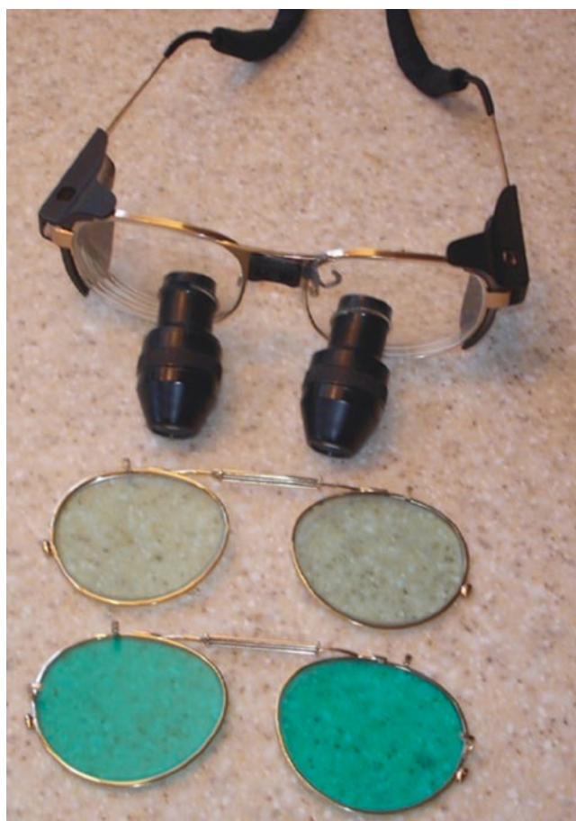
Fig. 5.7 Example of surgical loupes with wavelength-specific inserts, designed to fit on the inner aspect of the eyewear between the loupe lens and the operator's eye. Picture courtesy Dr. D. Coluzzi
